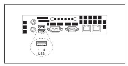
Figure 3-3. USB Connector Location and Pinout
